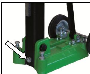
After drilling put the column back in the 90°position.
