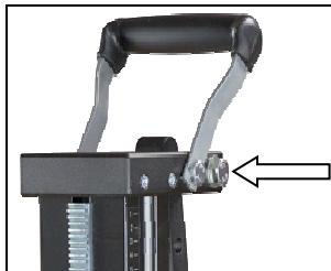
Open the top screw of the support with the turnstile.
