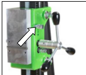
Move the machine holder upwards until it locks in the top position.
