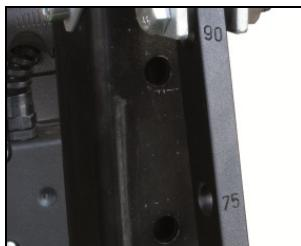
The different adjustable tilt angles are marked on the column.
