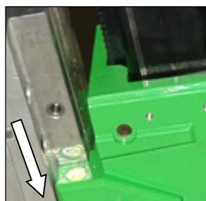
Insert the core drill with the attached mounting plate into the drill rig and lock it with the turnstile .
