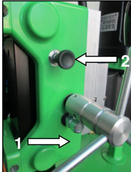
To unlock the carriage (1) pull out the lock knob (2).
