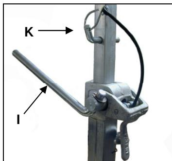
Fix the drill rig by turning the crank (L) clockwise. Secure in position by means of the appropriate bolt (K).
