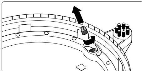
1. Unscrew the nozzles from the bracket on the cleaning rotor.
