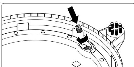
4. Rinse high-pressure hose and cleaning rotor. Screw in nozzles again. Use teflon tape for sealing. ... and you can proceed with the high-pressure cleaning as before !
