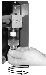
9) Kondensatbehälter passgenau eindrehen Turn the condensate tank accurately in
