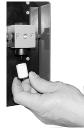
7) Filter einsetzen Set the filter in
